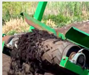
Machinery turns and mixes the piles, incorporating air that helps in the decomposition process. Temperature and moisture are carefully monitored, ensuring that the natural process can unfold regardless of weather conditions.
